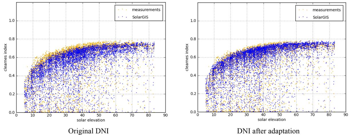
**FIGURE 2.** Clearness index vs. solar elevation for original and site-adapted SolarGIS DNI (Stellenbosch, South Africa). Left: original, right: site-adapted data.
